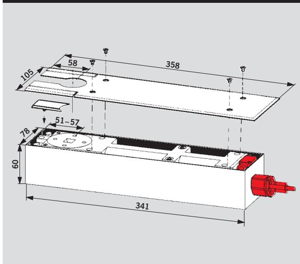
Floor spring with free-swing feature (electro-hydraulically controlled spring detent)
